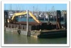
110 ton Komatsu Longreach Excavator Fitted with Trimble System
