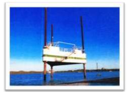
**"PLB1"** Piling Barge with 25T crane
